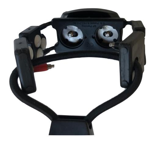
Place the receiver such that the posts for the contacts fit through the holes in the center piece of the Extender with the posts of the receiver facing to the inside of the Chameleon® Extender.
