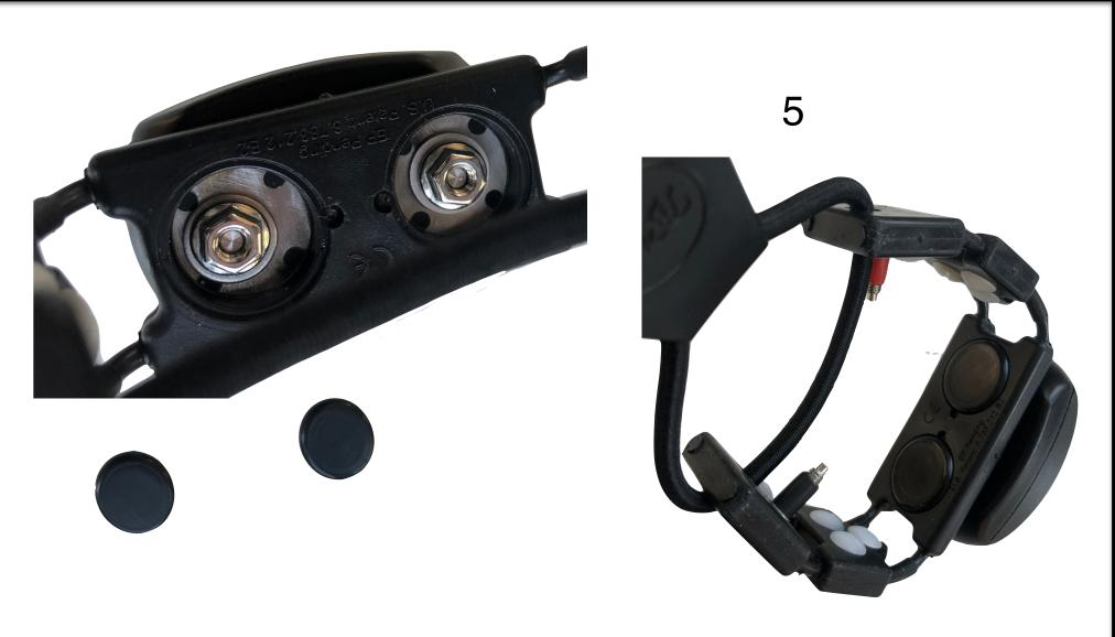
Tighten the washers and bolts, and then replace the covers on the back of the CEMS®.
